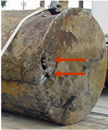
These corrosion holes were documented in a UST that was removed in Lebanon, Ky.
